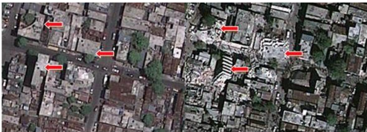
Figure 74: Pre- (left) and post-event (right) imagery of "pancaked" and "stair-step" damage patterns
