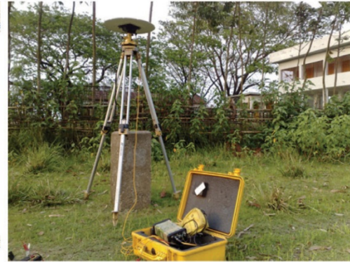
Setting coordinates for reference points in images using GPS technology
