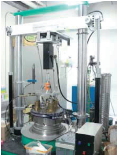
Fig. 3. The front view of the pore-water-pressure control ring shear apparatus (DPRI-7).
