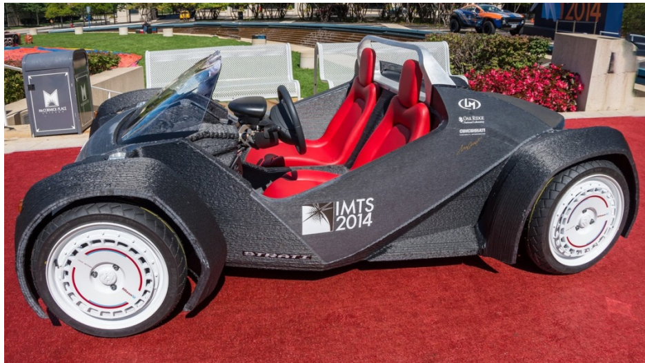
Figure 5.4. Local Motors 3D printed car body
