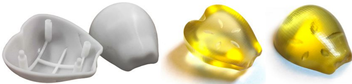
Figure 5.2. SLA (left) and PolyJet (right) printed parts
