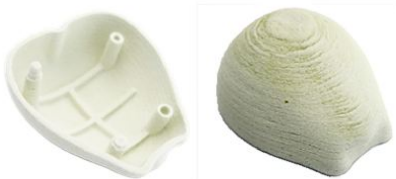
Figure 5.1. Experimentally printed part via ink jet
