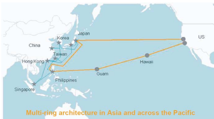
Figure 2-1c. A multi-ring architecture, reducing dependency on any one potential failure route 3
