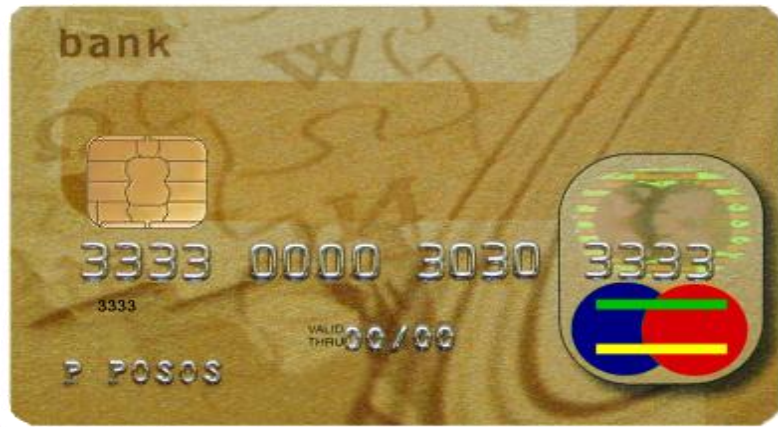
Figure 21 : A smart card, combining credit card and debit card properties. The contact pads on the card enable electronic access to the chip.
