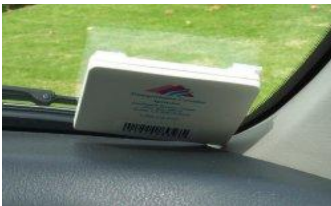
Figure 16 : An RFID tag used for electronic toll collection
