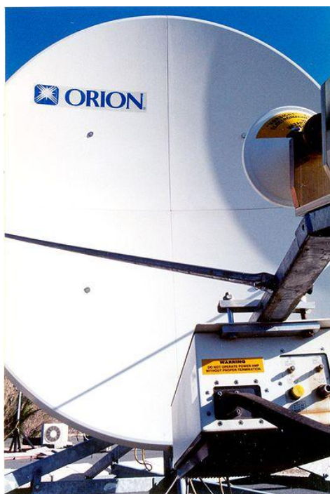
Figure 25 : A VSAT terminal
